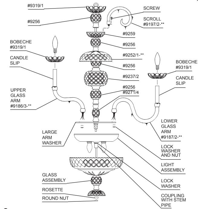
Install scrolls into washer with screws provided. Install arms into large arm washer. Line up holes in arms with dimple in washer. Use lock washer and nut to secure arms in place. NOTE: 6 Upper arms into inside diameter holes and 12 lower arms into outside diameter holes. Connect bare ground wires in each arm to bare ground wire in center column. Use electrical tape to secure wire nuts. NO MORE THAN 5 - WIRES PER WIRE NUT. Sufficient quantities of jumper wires and wire nuts are provided.
