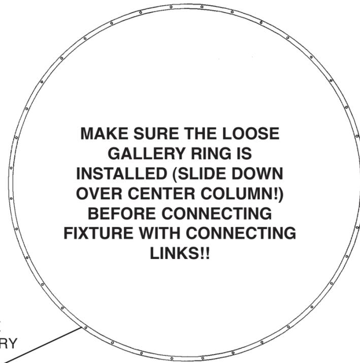
**23** Hook Chains "A" into the top inside ring pin holes. Hook the other end into the loose gallery ring inside pin holes. NOTE: Small jewels on upper end with metal connectors facing outwards.
