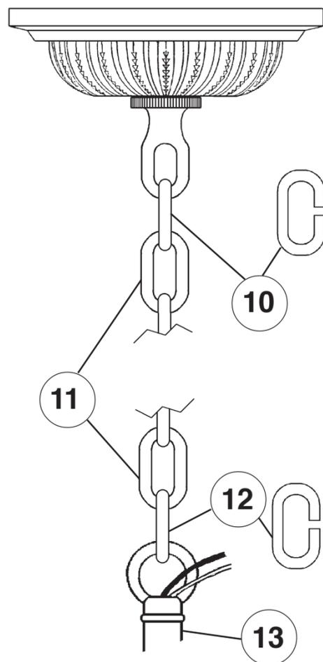
**MAKE SURE THE LOOSE GALLERY RING IS INSTALLED (SLIDE DOWN OVER CENTER COLUMN!) BEFORE CONNECTING FIXTURE WITH CONNECTING LINKS!!**
