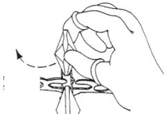
**27** Hook Chains "D" into the middle gallery ring #6. NOTE: Hold onto the square stone and turn chain side ways, this will allow connector to pass through slot in metal ring. Turn square stone to face the outside of the fixture and lower it until it seats itself in the ring. Hook the other end into the pin holes of the finial.
