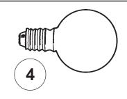
You will need 3 - G16-1/2 25 Watts Recommended 40 Watts Max MIN 90°C SUPPLY CONDUCTORS
