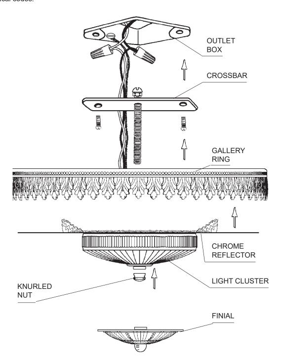
1 Remove crossbar from light cluster and reflector. Attach to outlet box in ceiling.
